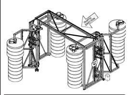
(2) FRONT BRUSHES "WRAP" TO CLEAN FRONT AND SIDES OF THE VEHICLE, (2) REAR BRUSHES "WRAP" TO CLEAN SIDES AND REAR SURFACES.
