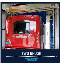
(2) side brushes apply friction cleaning to sides, front and rear surfaces. Dual nozzle, adjustable detergent spray bars are mounted on each side of the gantry. Water recycling system employs reclaimed wash water for rinse and under chassis wash functions.
