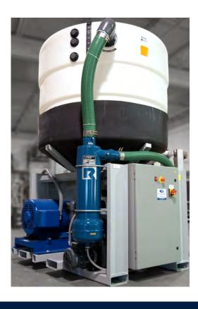
The modular design requires only 25 ft<sup>2</sup> of space allowing for easy installation using a reclaim pit and almost any site configuration
