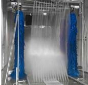
The Hybrid Wash System is a drive through wash system designed to use a combination of touchless cleaning for the front, top, wheel, under chassis and rear of a transit vehicle and foam brushes for the sides.
