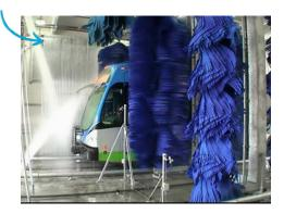
As the vehicle moves through the wash, sensors detect its position and activate the high-pressure touchless cleaning component, while also activating and deactivating the brushes.
