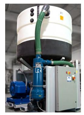
The modular design requires only 25 ft<sup>2</sup> of space allowing for easy installation using a reclaim pit and almost any site configuration
