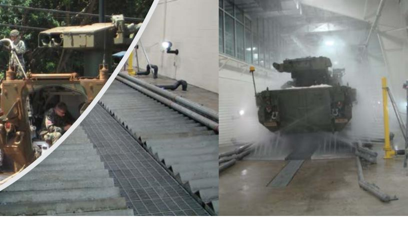
By using efficient and effective water recycling systems, InterClean is able to utilize the full force of high volumes of pressurized wash water. This creates a cleaning impact that is simply not possible with other vehicle washing systems.
